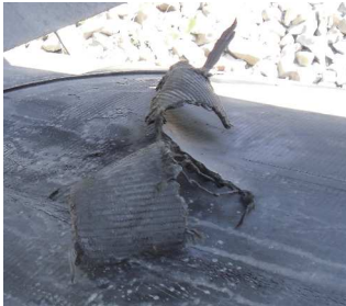
Before Repair : Large tear in belt due to rocks getting caught under the scraper blade.
