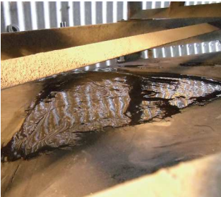
After Repair : Belt flap cut down, Devcon Surface Conditioner and R-Flex applied to belt.
